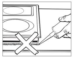
Under no circumstances should sealant find its way between the frame of the top part of the hob and the worktop.
